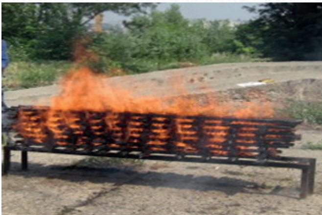
Figure 3 – Typical test fire class A
