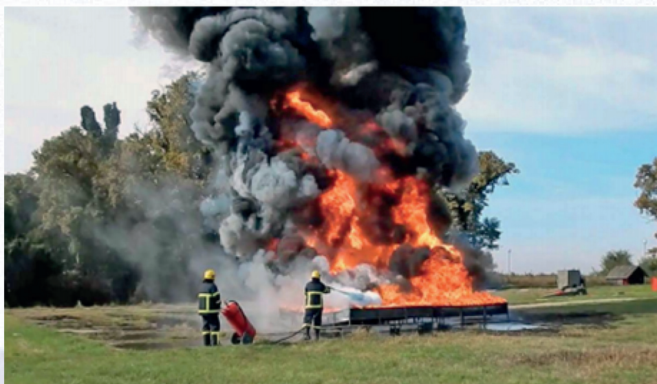
Figure 2 – Extinguishing fire at type B test fire
