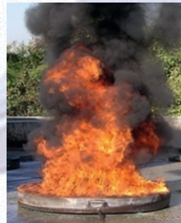
Figure 4 – Typical test fire class B
