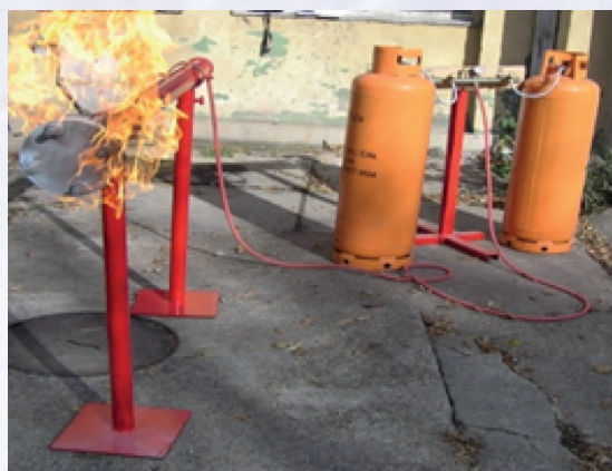
Figure 6 – Testing extinguishing at gas installations
